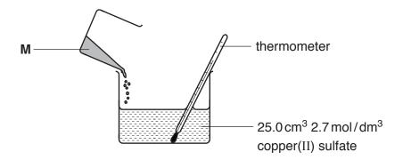
The student repeats the experiment using different masses of metal  ${\bf M}$  and in each case calculates and records the maximum temperature rise.
